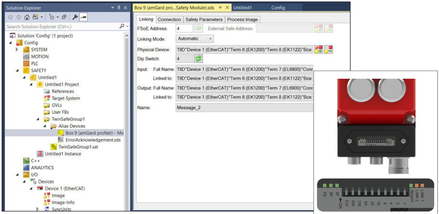
**NOTE:** The dip switch on amGard*pro pro*Net EtherCAT device reflects the FSoE Address of the module, it must be the same as the number entered within the safety project. The dip switch can be read in Free Run like above and the Fortress *pro*Net EtherCAT device will only update its value after a power cycle.
