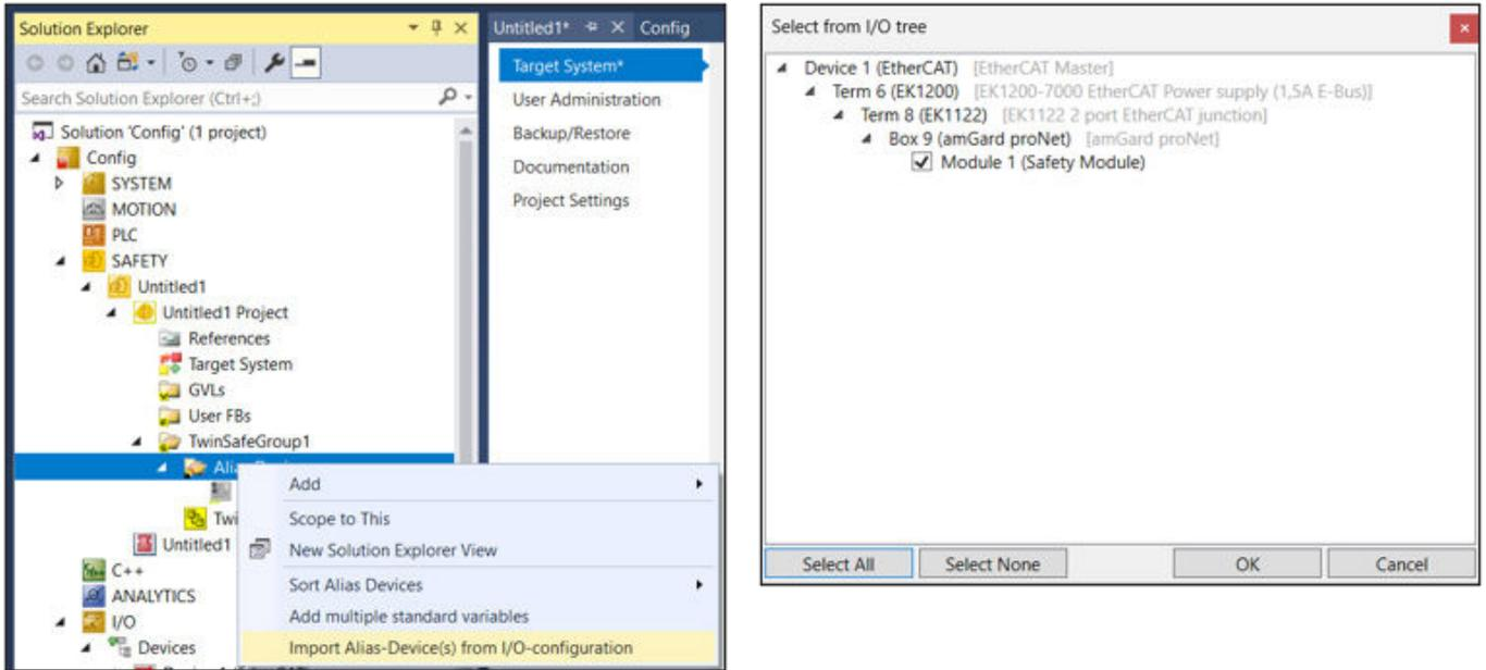
Select the amGard*pro pro*Net EtherCAT device under 'Alias Devices' to view device properties.
