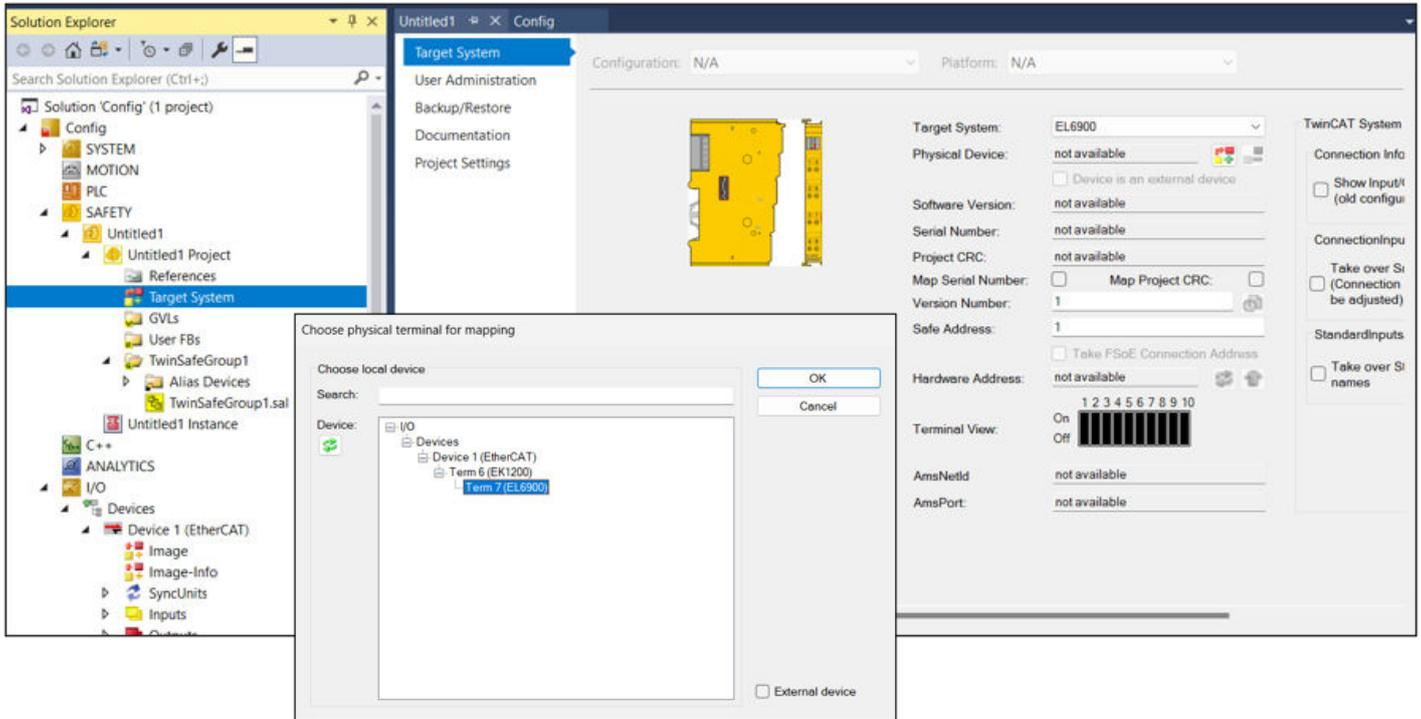
The Safe Address of the master needs to be set both on the device and in the safety project.
