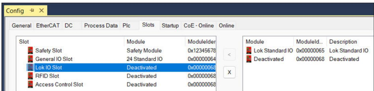
Before activating the configuration, any safety I/O modules need to be configured by creating a Safety Project.
