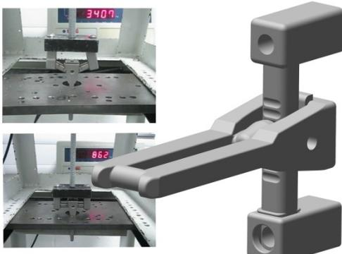
*Fortress' TA actuator remains intact beyond 4000 Kg of load; a typical actuator breaks around 700Kg*
